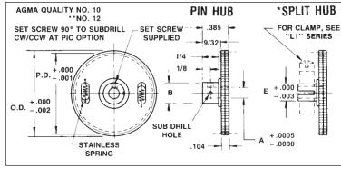
Gears — 303 Stainless Steel 2024-T4 Aluminum (Anodized Before Cutting)
