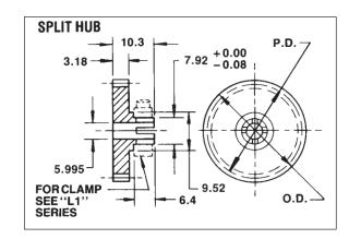
Material: 303 Stainless Steel 2024-T4 Aluminum (Anodized Before Cutting)
