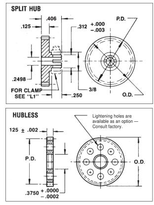
Material: 303 Stainless Steel 2024-T4 Aluminum (Anodized Before Cutting)
