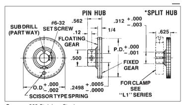
Gears — 303 Stainless Steel 2024-T4 Aluminum (Anodized Before Cutting) \*For split hub add -C to Part Number Pin Hub —  $\frac{1}{4}$ " Face Width =  $\frac{1}{4}$ " Bore = AGMA Quality No. 10
