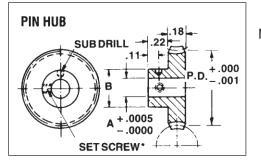
Material: Bronze QQ-B-637 Alloy 464 Ratio =  $\frac{\text{No. Teeth}}{\text{No. Threads}}$
