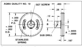
Gears — 303 Stainless Steel 2024-T4 Aluminum (Anodized Before Cutting) Hubs — 303 Stainless Steel
