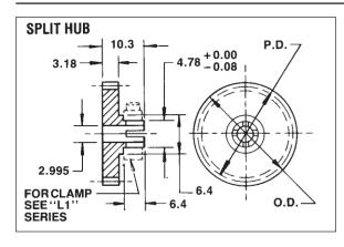
Material: 303 Stainless Steel 2024-T4 Aluminum (Anodized Before Cutting)
