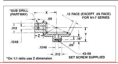
Material: 303 Stainless Steel — S 2024-T4 Aluminum (Anodized Before Cutting) — A
