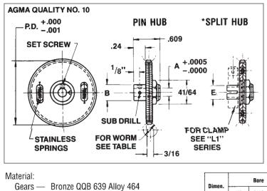
14<sup>1</sup>/2° Pressure Angle = Single, Double & Four Thread = Pin Hub — <sup>1</sup>/8", <sup>3</sup>/16" & <sup>1</sup>/4" Bores
