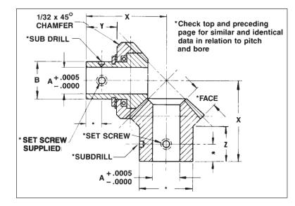
Gear Data Part No. No Per Set z Pitch Material P.D. B X Y A Teeth 36/36 S/A 500/.500 1248 1/4 .531 .185 .187 N1-1-AB 72 .187 N1-1-AB-S 36/36 S/S .500/.500 1248 1/4531 185 32/32 500/.500 17/64 562 .212 250 N2-1-AB S/A 1873 64 32/32 500/.500 1873 17/64 .562 .212 250 N2-1-AB-S S/S .312 N3-1-AB 30/30 S/A .625/.625 .2498 3/8 .687 .257 48 .312 N3-1-AB-S 30/30 S/S .625/.625 .2498 3/8 .687 .257
