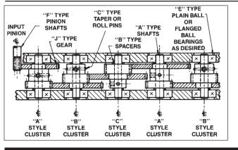
The following PIC cluster gears have been designed to allow large gear reduction. Quickly assembled with minimum space requirements.
