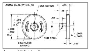
Gears — 303 Stainless Steel 2024-T4 Aluminum (Anodized Before Cutting)
