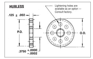
Material: 303 Stainless Steel 2024-T4 Aluminum (Anodized Before Cutting)
