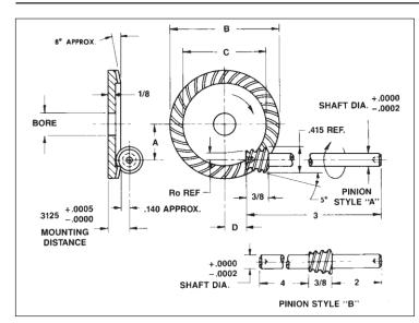
Material: Gears — Bronze ASTM B21, Alloy 464 Pinions and Hubs — 303 Stainless Steel
