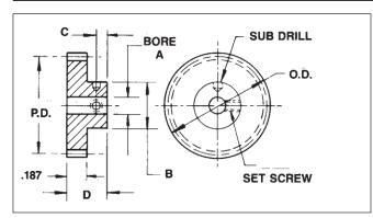
Material: 303 Stainless Steel 2024-T4 Aluminum (Anodized Before Cutting)
