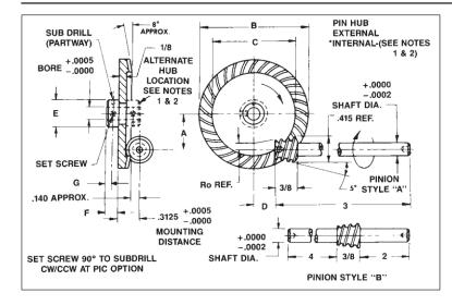
Material: Gears — Bronze ASTM B21, Alloy 464 Pinions and Hubs — 303 Stainless Steel
