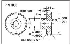
Material: Bronze ASTM B21 Alloy 464 Ratio = <u>No. Teeth</u> No. Threads
