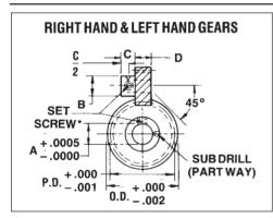
Material: 303 Stainless Steel 2024-T4 Aluminum (Anodized Before Cutting)
