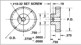
listing. Total Composite Tooth-to-Tooth Composite AGMA Quality Number 10-C .0010 .0007 Up to 20 Teeth Inclusive Over 20 Teeth-up to 1.999" P.D. .0005 .0010 Over 20 Teeth-2" to 2.999" P.D. .0005 .0012 Over 20 Teeth-4" P.D. and over .0005 .0014
