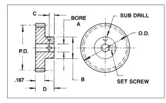
Material: 303 Stainless Steel 2024-T4 Aluminum (Anodized Before Cutting)
